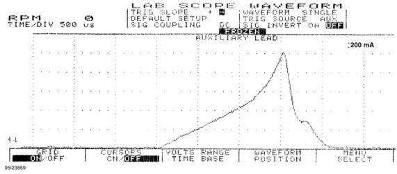
Fig. 14: Single Injector w/Normal Current Flow - Current Pattern
